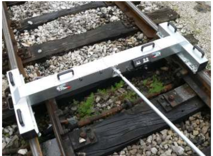
System configuration with two detection units in order to measure both the rails simultaneously
